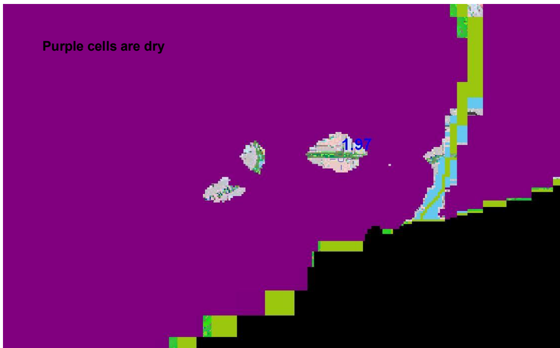
Figure 3-23 Target Residuals in Layer 1 (Made Ground) (figure zoomed into site area)
